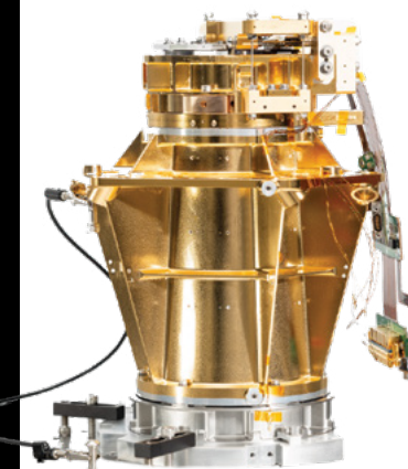
Right: State-of-the-art Dyson Imaging Spectrometer with MDL grating.
