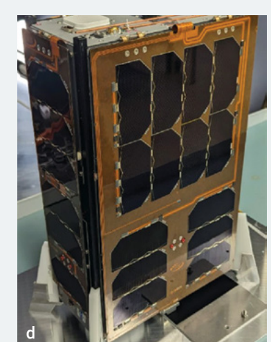
(c) HyTI 6U SmallSat; (d) ISISPACE 6U SmallSat, which could deliver 60 W peak power and a pointing accuracy of 0.1 degree; (e) SpaceX CRS-30 launch on March 21, 2024.
