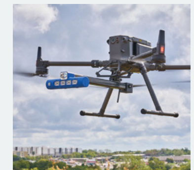
Methane leak detection with SeekOps drone-mounted sensor.
