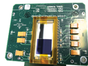
Sensor board and detector for the near UV channel of the SPARCam for SPARCS.
