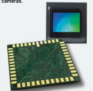
Aptina Imaging Corporation's 10-megapixel complementary metal-oxide semiconductor sensor is the first such device for point-and-shoot cameras.
