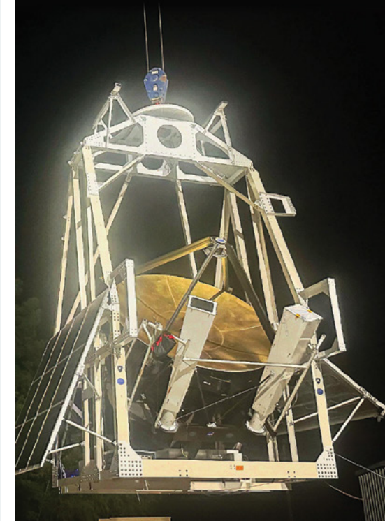
The ASTHROS mission's primary mirror is one of the largest to ever fly on a high-altitude balloon.
