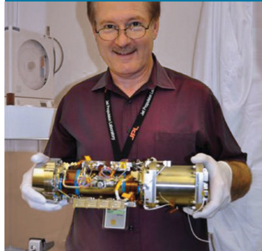
Dr. Webster holds a laboratory duplicate of the Mars TLS instrument to be used for testbed studies.
