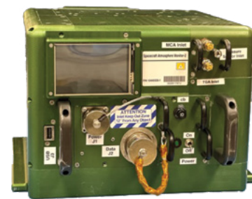
The TDU2 aluminum chassis is 9.5" x 8.75" x 7.5" in volume with a mass of 9.5 kg.
