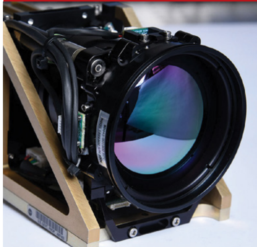
Handheld mid-wavelength infrared HOT-BIRD camera.
