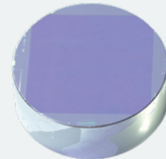
Above: SHERLOC contains a UV grating from MDL that produces excellent spectra with near-theoretical-maximum diffraction efficiency and negligible scatter.
